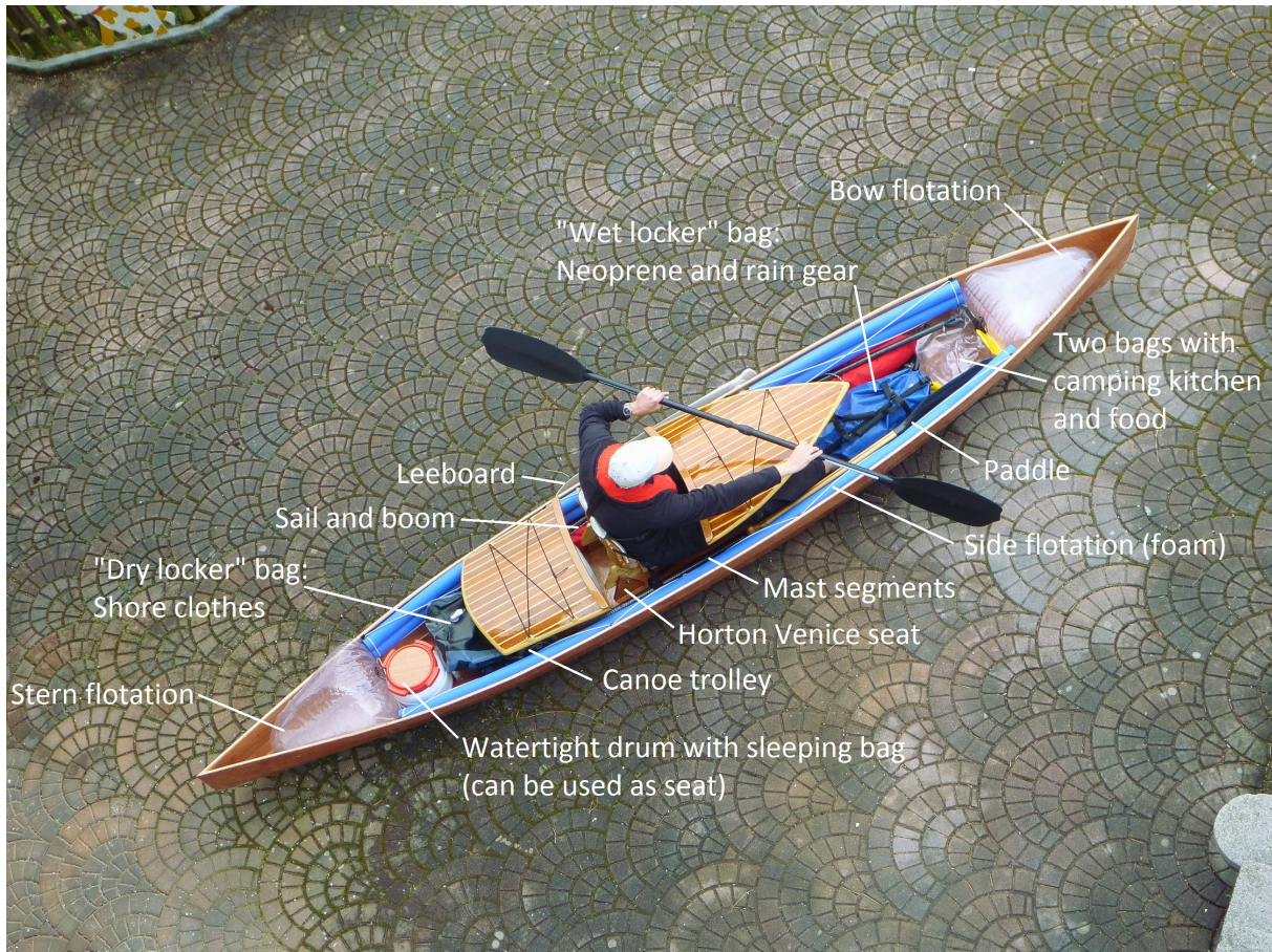
ARTEMIS without deck. I prefer this packaging layout for a cruise of several days.
