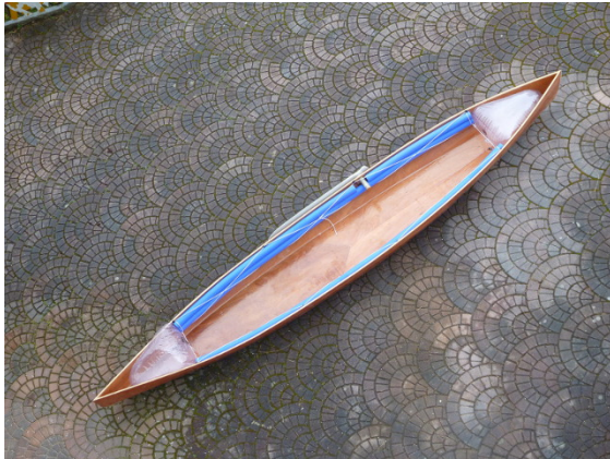
ARTEMIS without deck, showing bow, stern and side flotation
