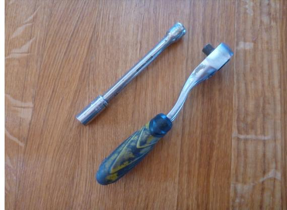
The small ratchet with extension and 7 mm socket is the only onboard tool you need. It is used to loosen and tighten the leeboard clutch mechanism. During the build, you are happy to have it for tightening the U-bolts at bow and stern from the inside of the boat.
