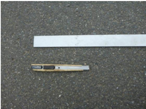
You cut fibreglass with the knife, and sometimes it is coated with epoxy. Therefore I have a knife with disposable blades that you can replace as needed. Use an aluminium ruler from the hardware store.
