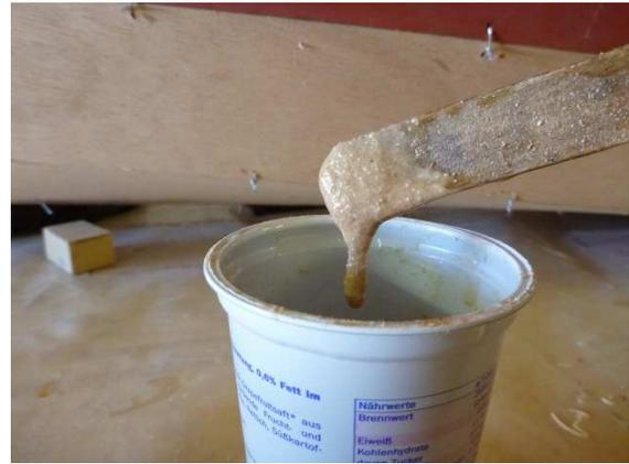
The splice is thinly coated with thickened epoxy. To prevent the glueing surfaces from sliding on one another, they will get staples on both sides. I staple them through some film, so that I can pull out the staples easily later...
