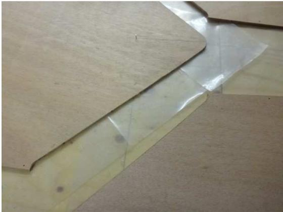
The plank segments are placed tightly together, the distances from the centreline checked once more. Then the plank segments are **weighted down so** that they **cannot slip**.
