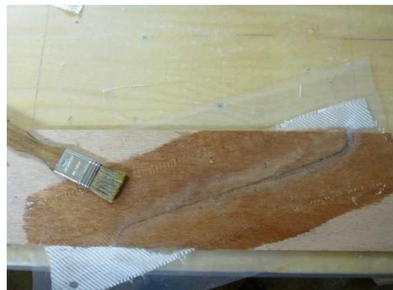
Put a strip of clear plastic film on top and wipe with your fingers the air bubbles between the film and glass fabric out to the side. A final check: Is the glass splice
