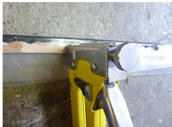
In the fore and aft bend, the film is stapled like a fan:
