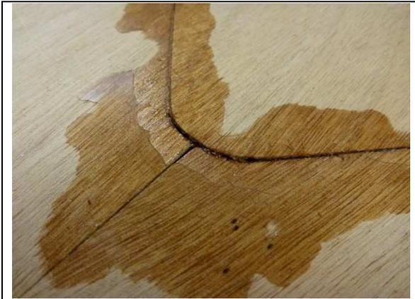
Here, the surface of the parts were not all matching and smooth across the surfaces before gluing. So, a step has formed on the outside of the planks. Because it is the bottom plank, one can plane the protruding segment smooth later and use some filler for the rest.
