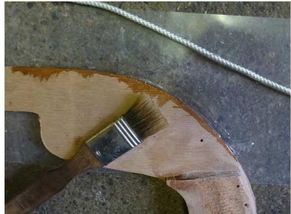
Wait until the epoxy just starts to thicken. The slightly longer than necessary glass cord is dipped in epoxy so that it is soaked. I have added some graphite powder to the epoxy – this will give an extremely hard and slippery surface. Apply glass cord ...
