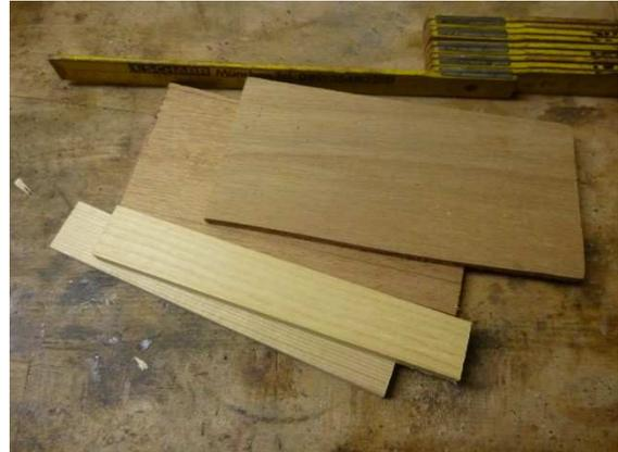
I nail these parts together so that a batten will run smoothly and without play through the gap in the middle. I nail some film in between the battens and the plywood - which gives a tad more distance, so the batten in the middle will run easier.
