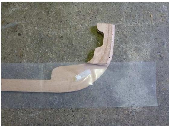
Then turn the skeg and apply epoxy resin onto the whole lower edge up to the skeg doublings:
