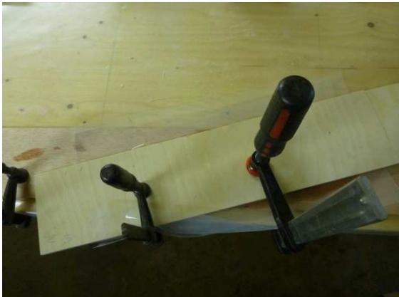
**Epoxy glue is space-filling.** If you bond epoxy with clamps, one can **only tighten them slightly**. The clamps should only press the glass fabric to the wood. If they would be tightened more, then one would force the epoxy out of the joint, no more epoxy would remain between the parts, and the connection would not be strong.
