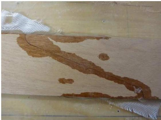
This bond looks clean and smooth on the outside. Some epoxy has seeped through the gap and has sealed it completely. Well done!
