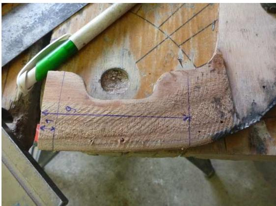
The top hole is 1 cm away from the top edge. The bottom hole is 9 cm from the top edge. Both holes are drilled parallel to the lower long skag edge.
