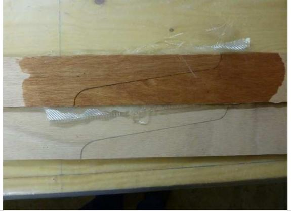
On the outside face I sand the splice of plank 1 slightly.
