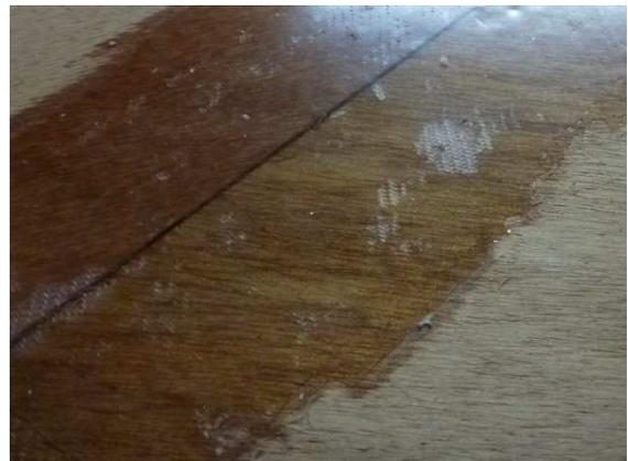
Here, not enough epoxy has been applied. Also, I have not completely pushed the air bubbles under the glass fabric to the side. So, some white spots are visible. The bond is generally sufficient. But the white spots will be noticed later when the boat interior is sheathed with fibreglass cloth and epoxy. So I'm going to sand out the white areas vigorously just prior to coating - but not until then! At the moment, I still need the entire load capacity of the seam.
