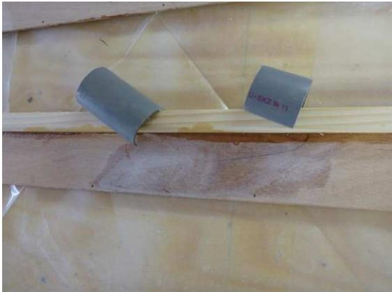
Remove epoxy oozing out of the joint before it hardens.
