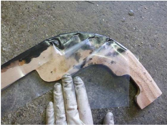
The picture shows that the glass cord at the rear end must go just around the curve up to the skag doublers, not all the way up.
