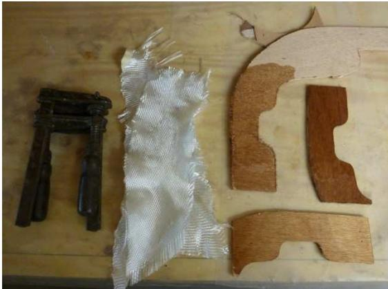
When the epoxy just begins to thicken, the glass weave strips are laid on the wood and some epoxy is brushed on them until they are transparent. These two could still use some epoxy:
