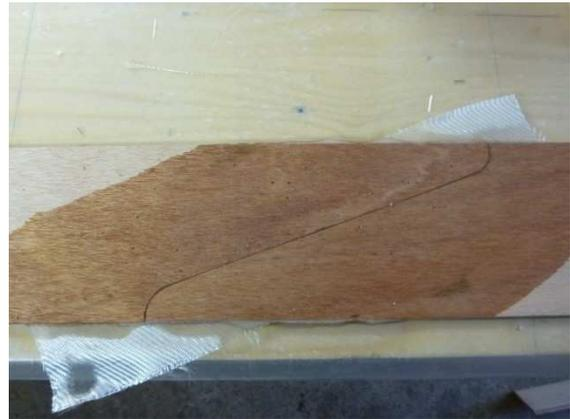
The splice should look like this on the inside. The parts are joined together without gaps. The bond is smooth, with no air bubbles or white areas.
