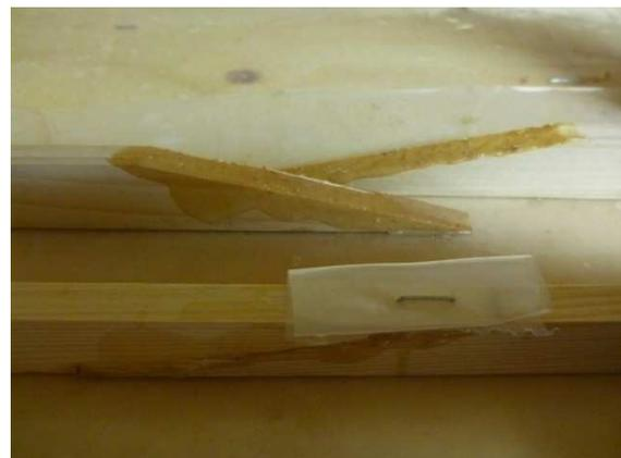
Before the gluing together, it is important to impregnate the wood with epoxy first.
