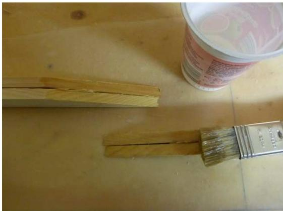
When the epoxy just begins to thicken, mix it with a little glueing powder. The thickened epoxy should just flow:
