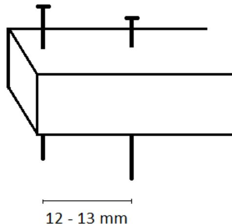
It is important to use about five clamps per stringer. They prevent slipping of the wet batten on the plank. In between, you can use spring clamps.
