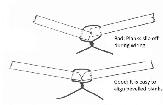
The chamfering with a few strokes by hand planing and finishing with some coarse sandpaper (60 grit or 80) is quickly done.
