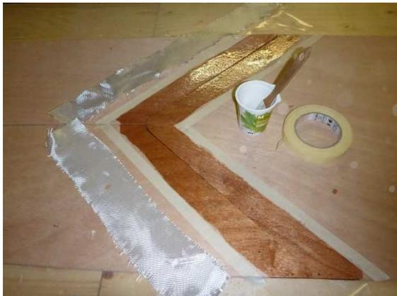
In the picture I did use painter's tape on the splices. Clear packing tape would have been better, because epoxy will not stick to packing tape.
