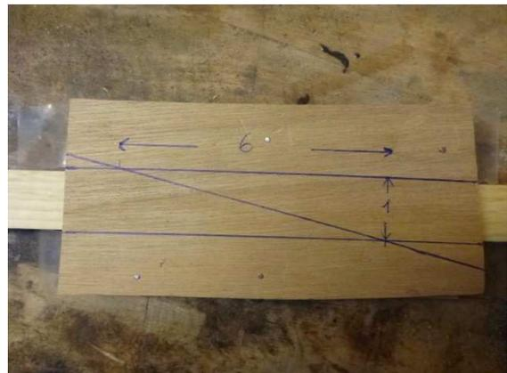
A scarf joint with epoxy is at least six times as long as wide. Clean, mark, insert, fix the batten in the gap and just saw along the line till the bottom wooden plate. Finished!
