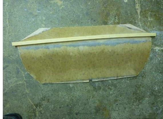
If you want a narrower boat, then the moulds B, C and D have to be cut slightly narrower at the contact surfaces to the plank 2, 3 and 4.
