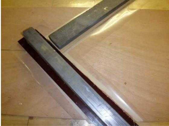
Place a waste timber over the splice and weigh it with a weight of about 10 pounds. A bucket or canister with water works well.
