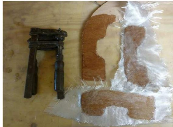
The laminates are then aligned with the skeg and secured against slipping with two spring clamps ...
