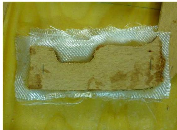
After drying, the front of the skeg is roughly cleaned with the rasp. The back is tapered on both sides with a planer and a rasp to create a good bonding surface for the planks: The depth is that both tapered faces will meet exactly at the centreline, where a ridge will form. Tapering should start about 20 mm away from that edge, so a total angle of about 35° is achieved. An angle which is too small would not hurt,
