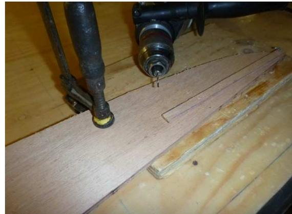
Drill the small holes with a sharp drill, high speed and low pressure, put underneath some waste timber. This will ensure that the holes will not fray.
