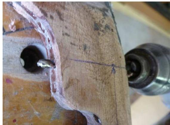
Drilling 4 mm holes through the skag is really easy, because the drill is guided by the glass weave between the skag faces. Anyway, ensure it does not overheat - then the epoxy would go soft. To prevent this from happening use a slower rotational speed and push somewhat stronger. Both of that will keep drill and hole cold.
