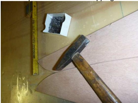
Then, prepare the plank segments for bonding: If the work surface is uneven, put a plate of scrap wood under the splice. One can then tack the plank segments down, to prevent slipping:
