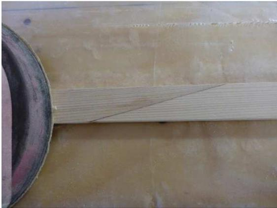
One of the four edges shall be rounded generously with a plane and sanding paper.
