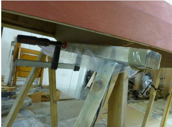
..., and check again with the two battens, clamped to the coaming, whether they are exactly parallel:
