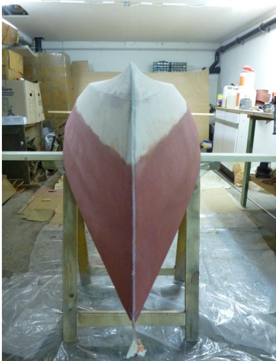
In the middle the 1.20 m long 9 x 18 mm batten under mould C ensures a good fairness of the bottom section:
