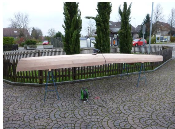
Rounding the edges I basically do by hand, with sandpaper on a small block.
