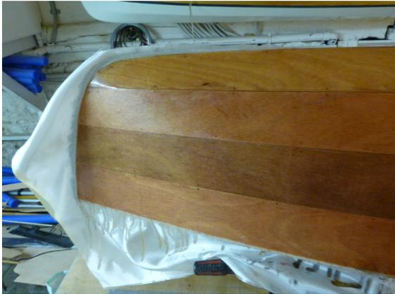
The fabric is cut a few inches before the skeg along the centre line so that the edge can lay flat on the hull.
