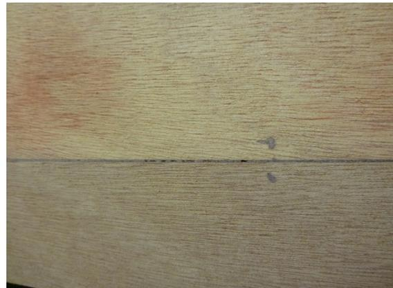
If you want to varnish the upper planks, it is important to not quite sand away the top veneer. At this edge the veneer of the inner layer is visible. This does not look very nice when it is varnished.
