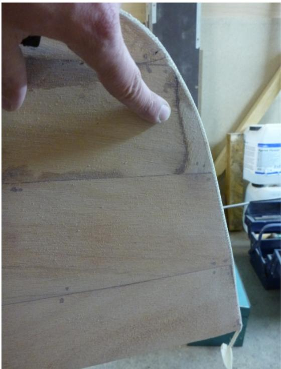
Then the machine comes back for the final sanding, this time with 120 or 180er sandpaper. At this stage I sand the entire surface silky smooth.
